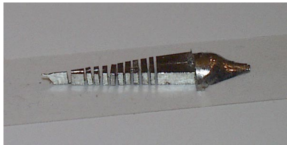
Figure 2.5: overview of wedge-shaped casting usage for sample preparation
