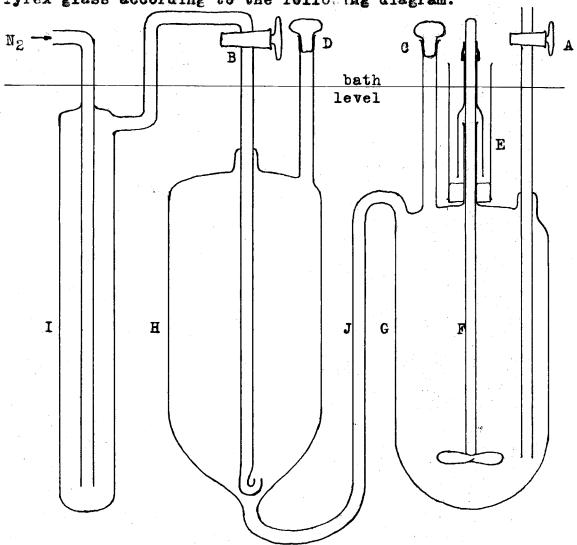
The apparatus was supported in the thermostat with the bath level at the point indicated. Nitrogen, previously passed through the glass bead saturator I filled with a solution of sulphuric acid prepared to approximate the
