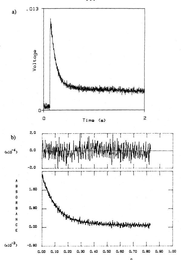
Figure 37. Flash-photolysis a) voltage/time and b) absorbance/time traces for 1  $\mu$ M Ru(H26)DP- $b_5$  (545 nm). Analysis using SI-FIT gave the fit shown and  $k_{obs} = 0.3 \text{ s}^{-1}$ .
