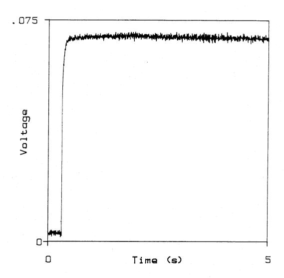
Figure 34. Flash-photolysis a) voltage/time and b) absorbance/time traces for 1  $\mu$ M Ru(H26)WT- $b_5$  (555 nm). The data in trace a) were converted to those in trace b) by T2A.BAS. Analysis of points from t = 0.4 to 1.6 s using SI-FIT gave the fit shown (inset is a plot of residuals) and  $k_{obs} = 2.2 \text{ s}^{-1}$ .
