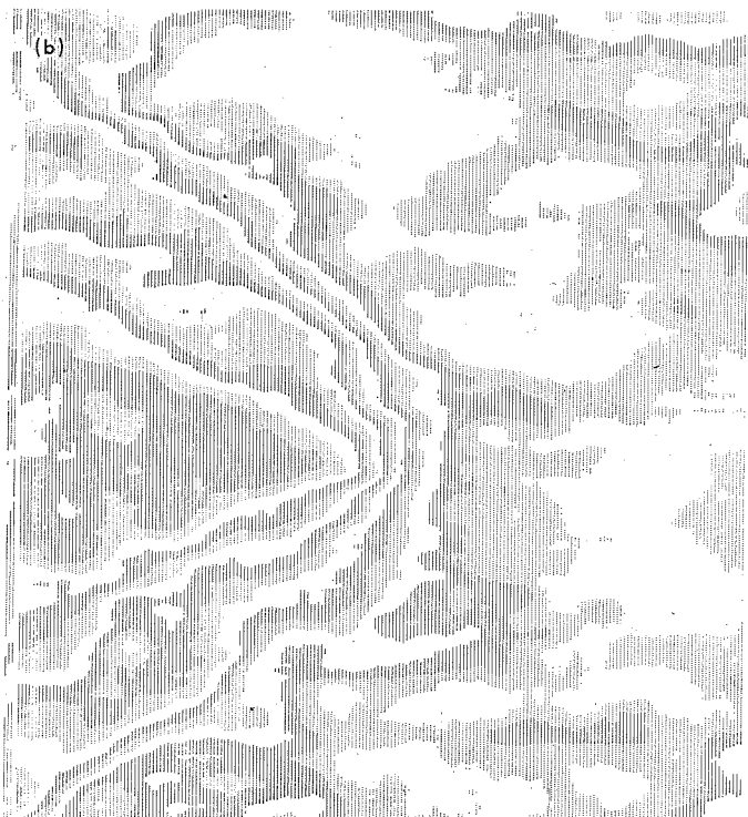
Fig. V-96. Isodensity tracings made from the negatives of supersonic flow over a 20° deflection wedge at M_1 = 4.0 ; \frac{1}{2} - \mu sec exposure [(a) tracing of 4 \times 5 negative; (b) enlargement of a Dynafax frame]
