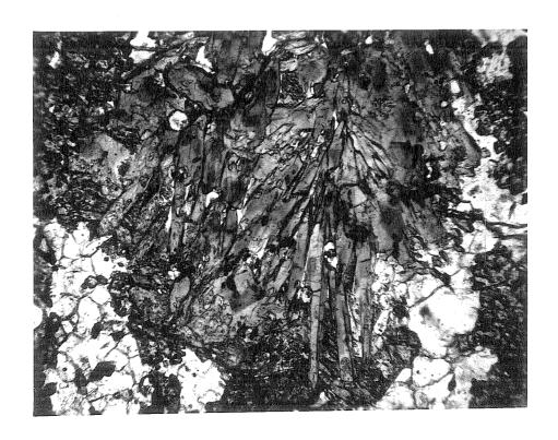
Pigure 7. Intermediate metamorphic grade feldspathic homblence schist with schistose homblende and biotite in a groundmass of quartz and plagioclase. (plain light, X54)
