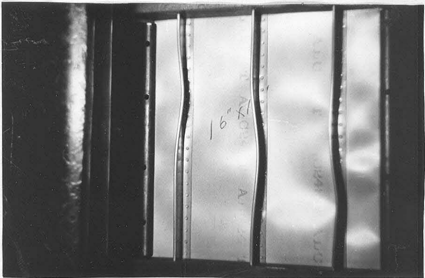
FIG VII TEST PANEL FAILED
