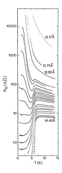
Fig. 1 Evolution of the temperature dependence of the sheet resistance R(T) with thickness for a Ga film [1].
