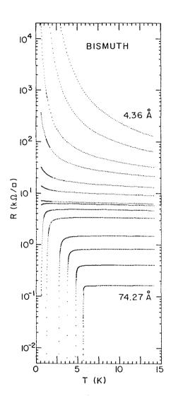
Fig. 2 Evolution of the temperature dependence of the sheet resistance R(T) with thickness for a Bi film deposited onto Ge [5].
