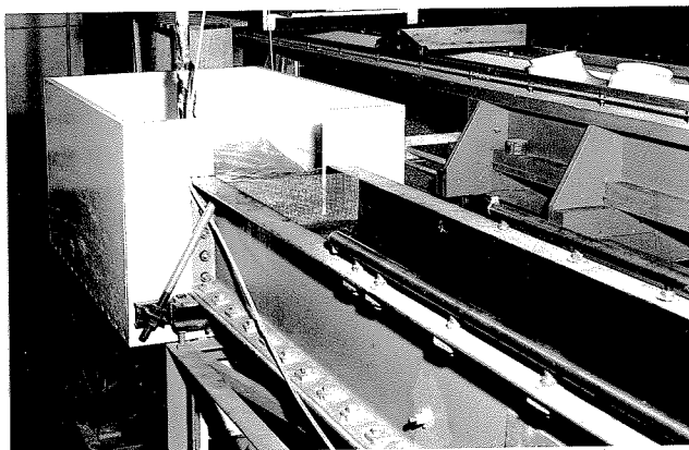
Fig. 3-5. Downstream end of 40-foot flume showing pump well used in Run Series 4.
