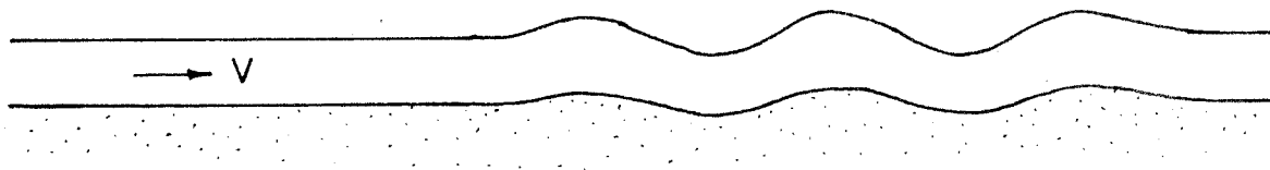
(b) Stationary waves and antidunes of figure (a) at time t_2 > t_1 . Note downstream propagation.
