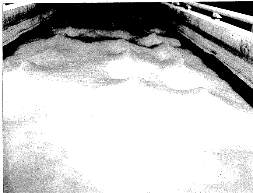
Fig. 4-4. Downstream view showing multiple trains of rooster tails. Run 4-11, d = 0.148 ft, V = 2.74 ft/sec, F = 1.26 , G = 16.6 lb/ft-min, f_b = 0.0397 , \lambda = 1.45 ft, 0.233 mm sand, 60-foot flume.
