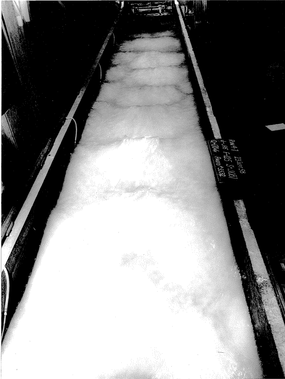
Fig. 4-2. Top view looking upstream showing growth of rooster tails from two-dimensional waves. Run 4-7, d = 0.195 ft, V = 3.14 ft/sec, F = 1.25 , 0.233 mm sand, 60-foot flume.
