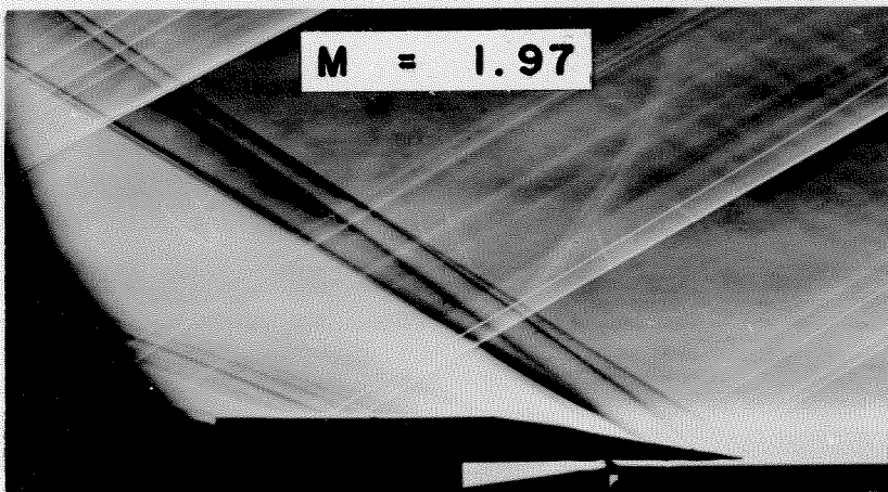
FIGURE 27. SCHLIEREN PICTURES OF THE A.C. GLOW PROBE IN SUPERSONIC FLOW
