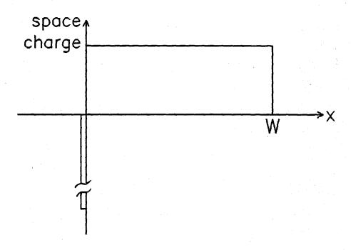
A being the diode area. If we add at x (0 < x < W) a small density n(x) of fixed negative charges in a region of width  $\Delta x$ , the depletion region will expand slightly, thereby uncovering more ionized donors — fixed positive charges — to compensate for the negative charges and maintain charge neutrality. The junction capacitance will drop by an amount  $\Delta C$ . It can be shown that this change is given by
