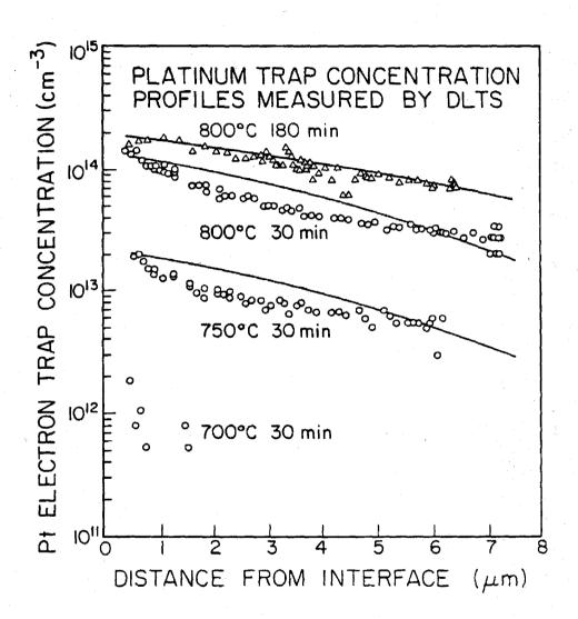
An extrapolation of the RBS data, discussed in Sec. 2.4.1, indicated that the platinum atom concentration falls off by an order of magnitude in 2000 Å (under the assumption that the RBS Pt tails were due to platinum at the interface). Since this fall off would correspond to an almost vertical line on the plot of Fig. 2.10, it is clear that the extrapolation of the RBS data is meaningless in the region of the DLTS measurements.
