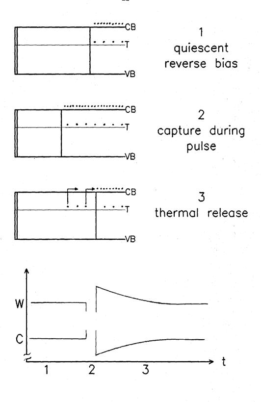
will then be positive. Thus, the sign of the transient is negative for an electron trap and positive for a hole trap. In general, the sign of the transient is negative for a majority carrier trap and positive for a minority carrier trap, regardless of whether the material is n- or p-type.
