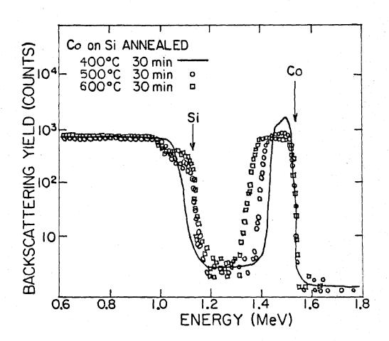
from the 600 °C case. No silicide formation was apparent in the 400 °C spectrum. Analysis yielded surface silicide compositions consistent with CoSi for the cobalt sample annealed at 500 °C, and CoSi<sub>2</sub> for the higher temperature samples. The low-energy fall-off of the cobalt signal did not appear to blur as temperature is increased.
