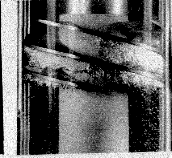
FIG. 22 CAVITATION DEVELOPMENT, IMPELLER ONE \Phi = 0.10 , RPM 6000
