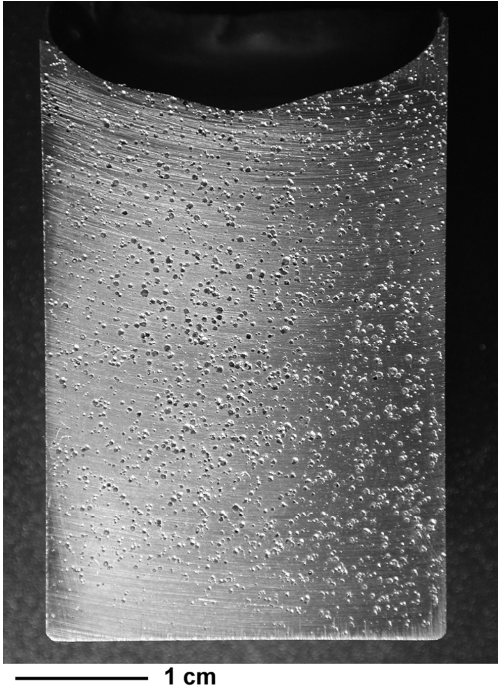
Figure 9. \text{Zr}_{58.5}\text{Nb}_{2.8}\text{Cu}_{15.6}\text{Ni}_{12.8}\text{Al}_{10.3} prefoam synthesized by the mechanical air entrapment method. It consists of 10-vol% bubbles with an average size of 250 microns.
