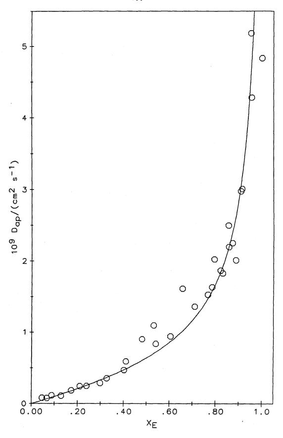
Figure 7.4. Comparison of experimental  $D_{ap}$  vs.  $X_E$  data (circles) with a theoretical curve (solid line) computed using  $\kappa=12$  (K=10 M<sup>-1</sup>),  $k_1=2.6\times10^6$  M<sup>-1</sup> s<sup>-1</sup>,  $\gamma=0$  ( $k_2=0$ ),  $\delta=1.4$  nm, and  $C_F^0=1.25$  M. Data were collected by Sharp and co-workers<sup>14</sup> using G<sup>+</sup>=Na<sup>+</sup> as the electroinactive counterion.
