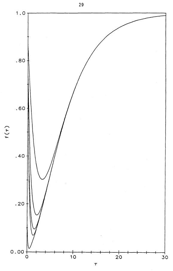
Figure 2.4. Fractional changes in current calculated from Equation 2.27. From the bottom to the top curve, M = 2, 4, 6, 8, and 10 exponential terms are utilized in the calculation, with S=1500 and  $\epsilon$ =-0.3. The last three curves are indistinguishable.
