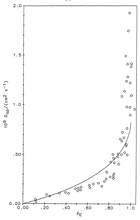
Figure 7.6. Comparison of experimental  $D_{ap}$  vs.  $X_E$  data (circles) with a theoretical curve (solid line) computed using the strong ion-pairing limit ( $\kappa$ >100),  $k_1/K=2.9\times10^4$  s<sup>-1</sup>,  $\gamma$ =7 ( $k_2$ =1.7 $\times10^5$  M<sup>-1</sup> s<sup>-1</sup>),  $\delta$ =1.4 nm, and  $C_F^0$ =1.25 M. Data were collected by Sharp and co-workers<sup>14</sup> using G<sup>+</sup>=Na<sup>+</sup> as the electroinactive counterion.
