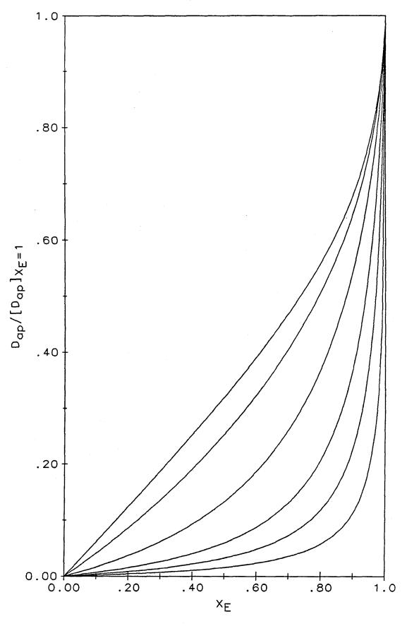
Figure 6.2. Variation of the apparent diffusion coefficient, normalized by its value at  $X_E=1$ , with the fractional loading for a coating loaded with  $Os(bpy)_3^{3+}$  with  $\gamma=0$ . The curves from bottom to top, i.e., those possessing the greatest to the least amount of curvature, are calculated using  $\kappa=10^5$ ,  $10^3$ , 100, 10, 1, 0.
