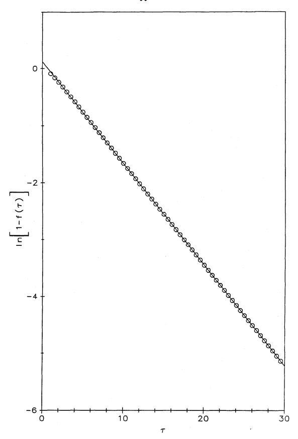
were derived. This agreement confirms that analysis of current transients resulting from the "magic" step change in rotation rate as simple exponential functions does not introduce significant error in the values of the Schmidt number obtained.
