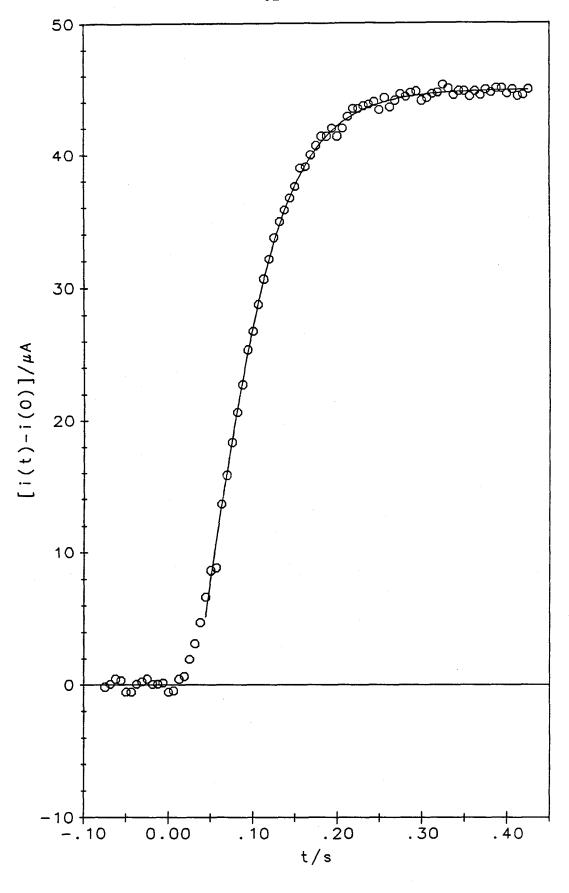
Schmidt number obtained from the least-squares fit corresponds to  $D=(6.8\pm0.2)\times10^{-6}~cm^2~s^{-1}$  and is in reasonable agreement with the accepted value for  $Fe(CN)6^{4-}$  in 1 M KCl at 25°C,  $D=6.33\times10^{-6}~cm^2~s^{-1}$  (S=1352). This agreement and that of the calculated line with the experimental points in Figure 4.1 indicate the reliability of Equation 4.1 and the orthogonal collocation procedure that produced it.
