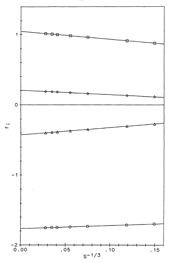
Figure 2.2. Variation of the first four collocation coefficients with the magnitude and sign of the change in rotation rate for a Schmidt number of 1500. Smooth curves were drawn through the calculated points. ( $\bigcirc$ )  $f_1$ ; ( $\square$ )  $f_2$ ; ( $\triangle$ )  $f_3$ ; ( $\diamondsuit$ )  $f_4$ .
