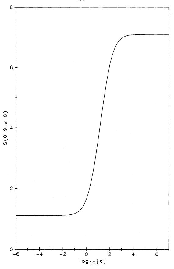
Figure 6.10. Variation of  $S(0.9,\kappa,0)$  with  $log_{10}[\kappa]$  for coatings loaded with  $Os(bpy)_3^{3+}$ .
