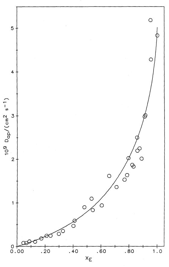
Figure 7.3. Comparison of experimental  $D_{ap}$  vs.  $X_E$  data (circles) with a theoretical curve (solid line) computed using the strong ion-pairing limit ( $\kappa$ >100),  $k_1/K=2.7\times10^5$  s<sup>-1</sup>,  $\gamma$ =2.2 ( $k_2$ =5.0 $\times10^5$  M<sup>-1</sup> s<sup>-1</sup>),  $\delta$ =1.4 nm, and  $C_F^0$ =1.2 M. Data were collected as part of this study using G<sup>+</sup>=H<sup>+</sup> as the electroinactive counterion.
