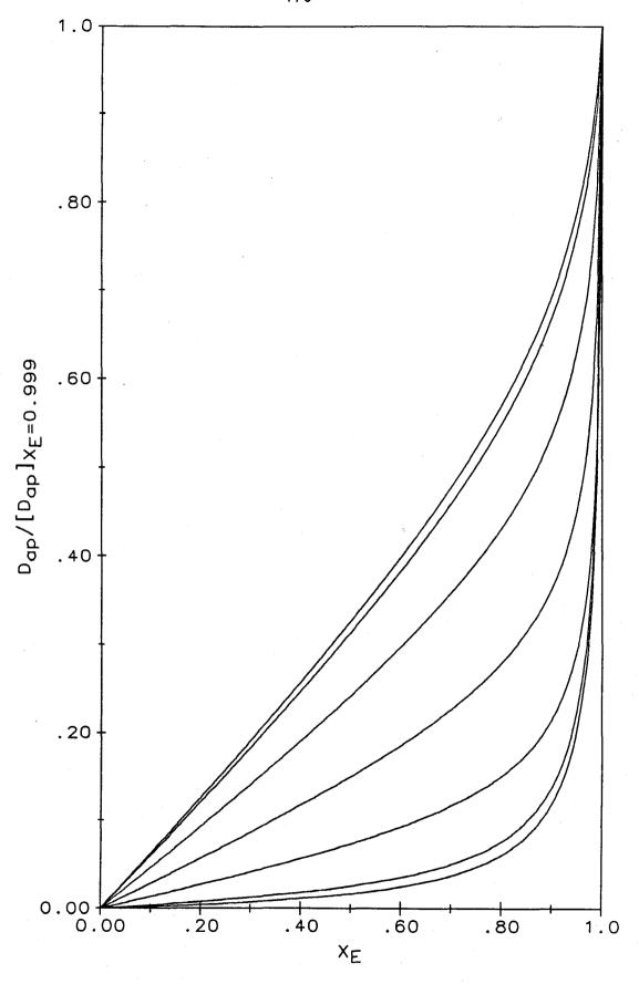
Figure 6.12. Variation of the apparent diffusion coefficient, normalized by its value at  $X_E=0.999$ , with the fractional loading for a coating loaded with  $Os(bpy)_3^{3+}$  in the strong ion-pairing limit, i.e.,  $\kappa>100$ . The curves from bottom to top, i.e., those possessing the greatest to the least amount of curvature, are calculated using  $\gamma=10^6$ , 100, 30, 10, 3, 1, 0.
