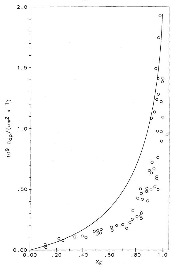
Figure 7.5. Comparison of experimental  $D_{ap}$  vs.  $X_E$  data (circles) with a theoretical curve (solid line) computed using  $\kappa=1.6$  (K=1.3  $\underline{M}^{-1}$ ),  $k_1=5.2\times10^5$  M<sup>-1</sup> s<sup>-1</sup>,  $\gamma=0$  ( $k_2=0$ ),  $\delta=1.4$  nm, and  $C_F^0=1.25$   $\underline{M}$ . Data were collected by Sharp and co-workers<sup>14</sup> using G+=Na+ as the electroinactive counterion.
