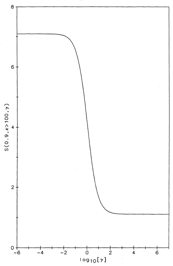
Figure 6.14. Variation of  $S(0.9,\kappa>100,\gamma)$  with  $log_{10}[\gamma]$  for coatings loaded with  $Os(bpy)_3^{3+}$ .
