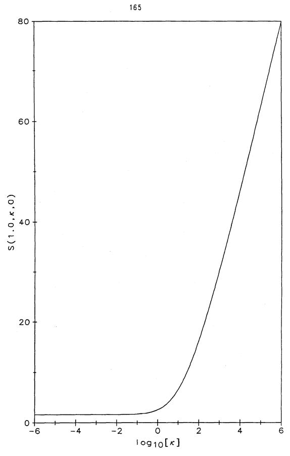
Figure 6.8. Variation of  $S(1.0,\kappa,0)$  with  $log_{10}[\kappa]$  for coatings loaded with  $Os(bpy)_3^{3+}$ .
