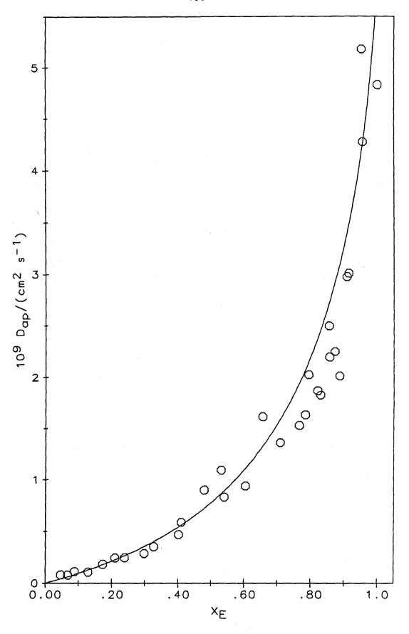
Figure 7.2. Comparison of experimental  $D_{ap}$  vs.  $X_E$  data (circles) with a theoretical curve (solid line) computed using  $\kappa=6$  (K=5  $\underline{M}^{-1}$ ),  $k_1=5\times10^6$  M<sup>-1</sup> s<sup>-1</sup>,  $\gamma=0$  ( $k_2=0$ ),  $\delta=1.4$  nm, and  $C_F^0=1.2$   $\underline{M}$ . Data were collected as part of this study using G<sup>+</sup>=H<sup>+</sup> as the electroinactive counterion.
