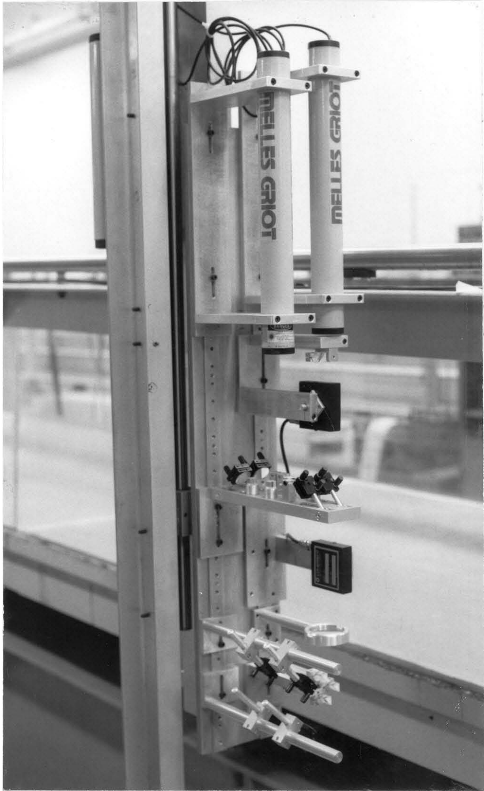
Fig. 4.11 Photograph of the LDV's transmitting optics.
