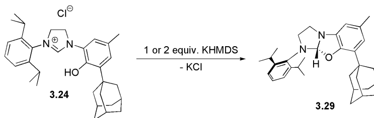
Scheme 3.12. Synthesis of cyclized product 3.29 by reaction of 3.24 with KHMDS.
