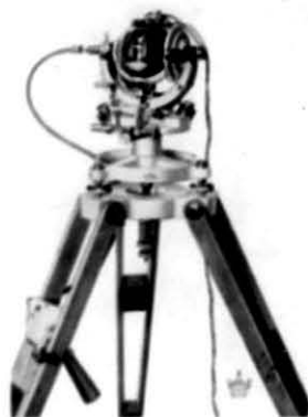
Fig. 6 Small Earth Inductor Rotating the coil in the earth's field induces current which is measured with a galvanometer having a sensitivity of 1 \times 10^{-9} amperes.
