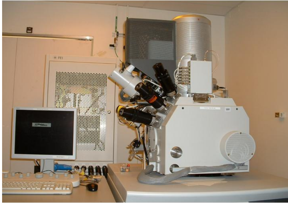
Figure 1.3: FEI Dual Beam Focused Ion Beam Nova 600: One of the two Nova system located in the KNI cleanroom
