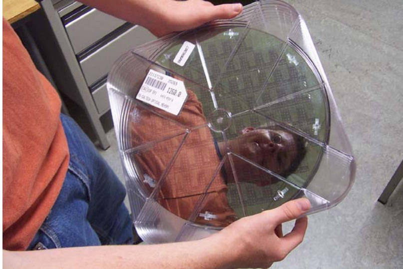
Figure 3.4. Silicon nanocrystal optical memory test devices fabricated on a 300 mm substrate at Intel.
