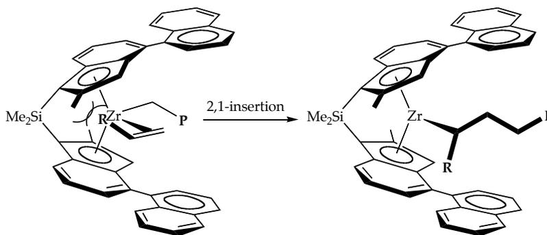
**Figure 3.** The 2-methyl substituents discourage 2,1-insertion of propylene by unfavorable steric interactions (**R** = alkyl, **P** = polymer chain).
