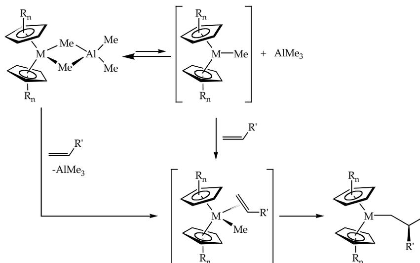
This study could enable a correlation to be made between ancillary ligand substitution, polymer molecular weight, and relative rates of the fundamental reactions that occur in the course of group 4 metallocene-catalyzed  $\alpha$ -olefin polymerization. Ultimately, this knowledge may allow for tailoring of catalysts to produce polymers of desired molecular weight.
