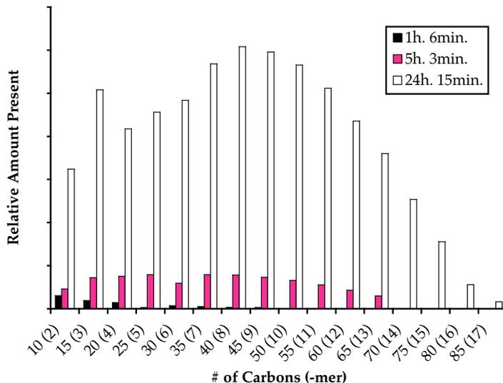
**Figure 8.** Relative amounts of oligomers of 1-pentene formed by catalyst **1** at different time intervals.
