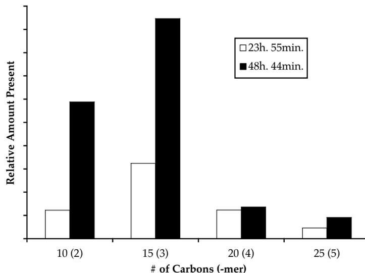
**Figure 10.** Relative amounts of oligomers of 1-pentene formed by catalyst 3 at different time intervals.
