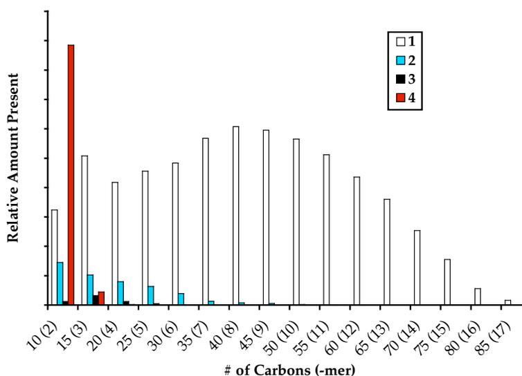
**Figure 11.** Relative amounts of oligomers of 1-pentene formed by catalysts 1-4 after 24 hours.
