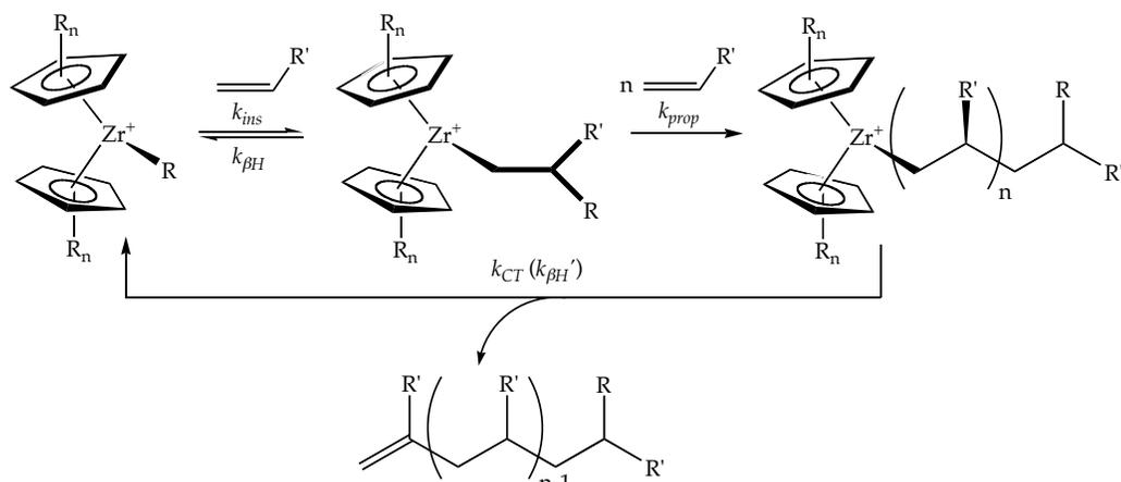
**Figure 1.** Fundamental steps in metallocene-catalyzed  $\alpha$ -olefin polymerization ( $R = H$ , alkyl;  $R' = \text{alkyl}$ ).
