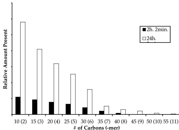
**Figure 9.** Relative amounts of oligomers of 1-pentene formed by catalyst 2 at different time intervals.
