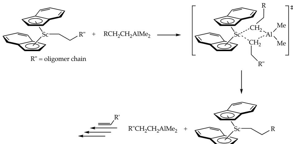
Catalyst **2** produces oligomers from dimer to undecamer (55 carbons). Unlike **1**, **2** produces a Flory-Schulz distribution of oligomers, which remains the same at different reaction times, indicating that oligomers that have been formed and eliminated do not reinsert (Figure 9). Thus, over time the same range of oligomer molecular weights is observed with greater amounts of each oligomer being produced at longer reaction times.
