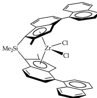
**Figure 2.** Spaleck's dimethylsilyl*bis*(2-methyl-4-naphthyl-indenyl)ZrCl<sub>2</sub> catalyst produces polypropylene of extremely high molecular weight.
