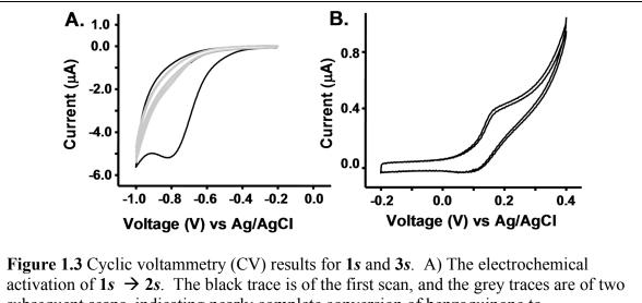
subsequent scans, indicating nearly complete conversion of benzoquinone to hydroquinone during the first scan. B) The reversible oxidation of **3***s*. Two subsequent scans are shown. All voltages are relative to Ag/AgCl.
