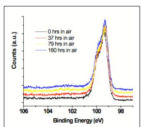
**Figure 1.1** XPS data of H-C=C-[Si(111)], collected in the Si 2p region, and taken after exposure to air for up to 160 hours. The peaks for SiO<sub>x</sub> species should appear between 100 and 104 BeV. The amount of oxidation of the Si(111) can be estimated from this data to be < 0.25 equivalent monolayers. The Si 2p features are normalized to the same height for all three scans. The 37, 79, 160 hours scans are shown offset from the 0 hours scan to reveal the spectral detail.
