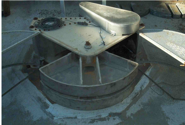
Figure A:4. Kinometrics VG-1 Synchronized Vibration Generator (Shaker). The counter-rotating buckets, shown empty, can be loaded with different configurations of lead weights. The shaker is located on the roof of Millikan Library, as shown in Figure A:2.
