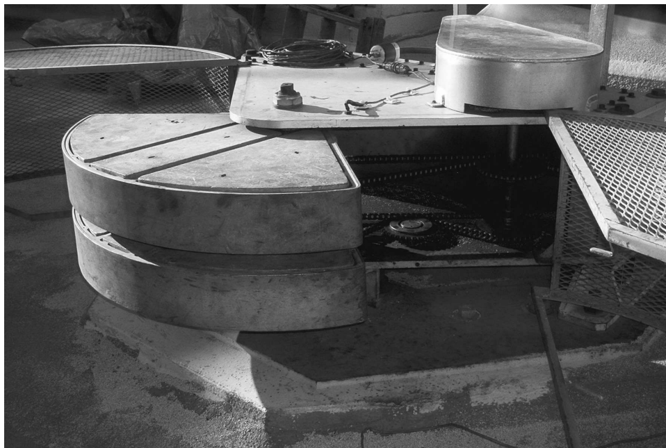
Figure 2.1 Picture of the force generating mechanism used to shake Millikan Library. The shaker is pictured here with full buckets (exerts maximum force).
