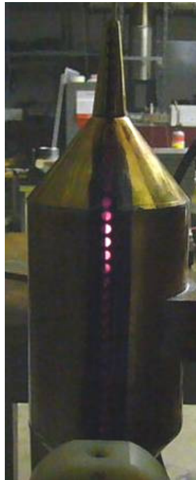
Fig. 7-6: Steady state microwave heating of a mullite tube (no flow).
