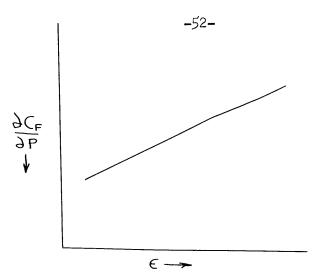
This plot will obviously show a linear relationship, and hence  $\frac{\delta^C_F}{\delta^P} = -\kappa_3 \in C_F$  can now be expressed as a function of  $\epsilon$ . Using the desired rocket parameters  $I_{\rm sp}$ ,  $\kappa$ ,  $a_{\rm o}$ ,  $v_{\rm o}$ , and  $P_{\rm c}$ , in conjunction with existing charts, 1-JD-92, the following plot is made:
