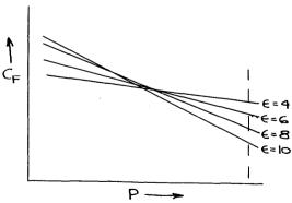
For each assumed value of  $\epsilon$ , determine the slope of this plot,  $\frac{\delta^{C_F}}{\delta^{P}}$ , and then a plot as made of  $\frac{\delta^{C_F}}{\delta^{P}}$  versus  $\epsilon$ .
