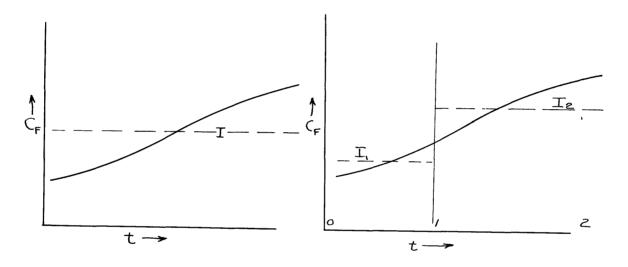
By this one-step approximation method, the upper portion of the flight pattern can be more justifiably weighted as against the poorer performance of the lower portion.
