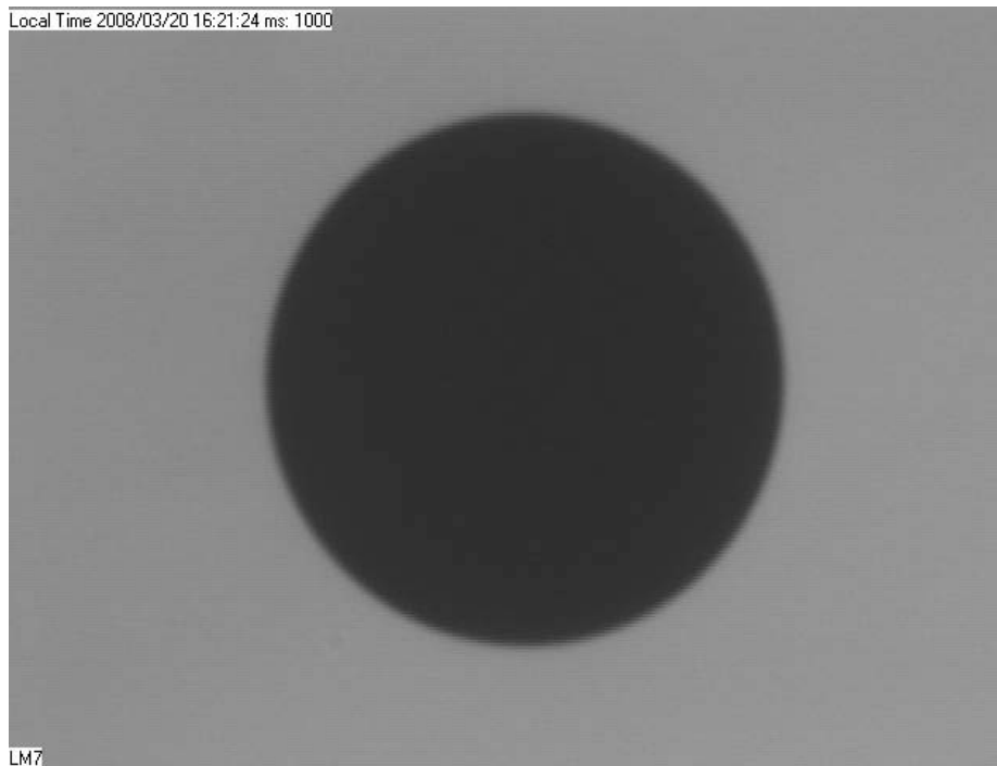
Figure 3.1: Backlight image of a molten Vit1 sample levitated in an ESL
