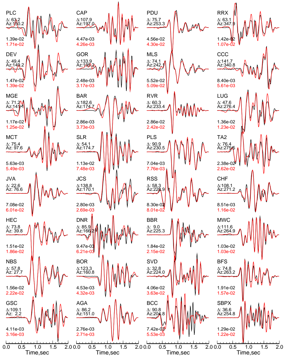
Figure 2.29: The records (vertical P waves) from event 13936432 (black) are compared with the “synthetics” (red) constructed from the EGFs assuming a uniform triangular (0.07–0.07 sec) source time function. A band-pass filter of 0.5–12 Hz has been applied. The amplitudes of the plotted traces are normalized by the maximum values given below the traces. Note the remarkable match between the shapes and amplitudes over the whole azimuthal range.
