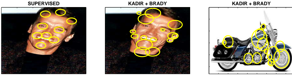
Figure 5.2: (Left) Examples of features selected manually for Schwarzenegger. Nine total features are selected. (Center) The same image but with features found using the Kadir and Brady detector. The 15 most salient features are shown.
