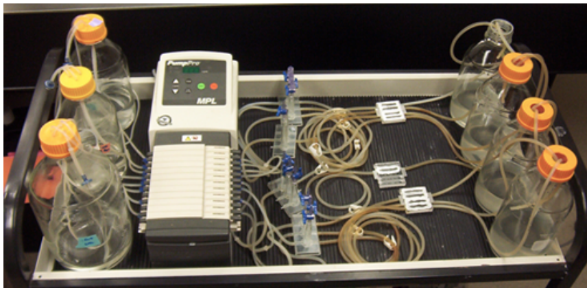
Figure A.1: Setup of biofilm once flow-through system on the biofilm cart.
