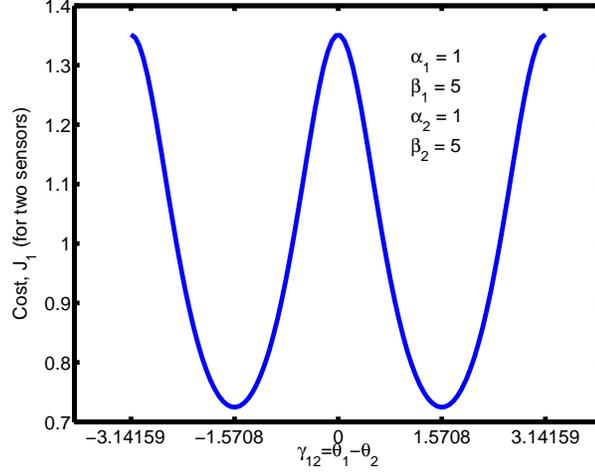
Figure B.1: Dependence of the cost function (for two sensors) on their relative bearings with respect to the target. This shows that in order to minimize the cost, the two agents should be separated by  $\pm \frac{\pi}{2}$  radians.
