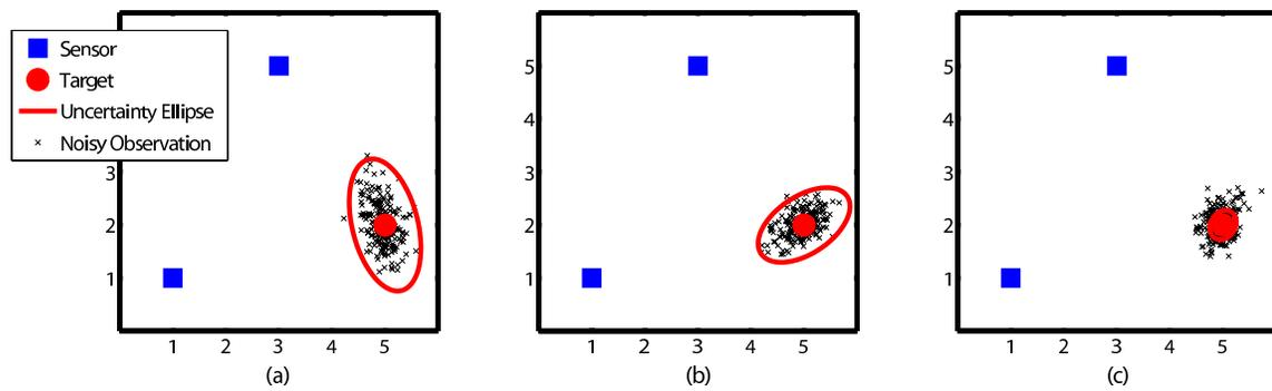
Figure 2.3: Illustration of the benefit of fusing multiple observations. Two (stationary) sensing agents make independent, noisy range and bearing observations of a planar target, which are fused to yield estimates with reduced uncertainty.
