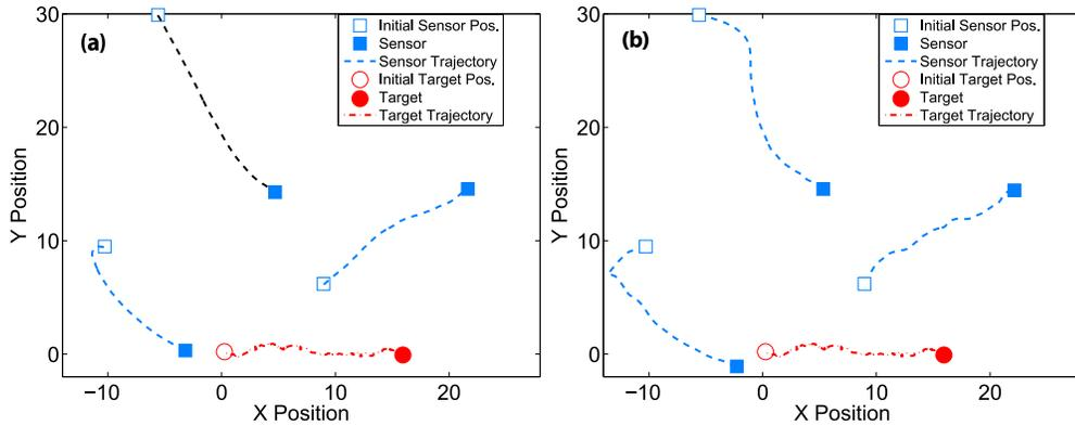
Figure 2.4: Three sensors track a (biased) randomly walking target using the proposed gradient-descent control law for costs (a)  $J_1$ , (b)  $J_2$ .
