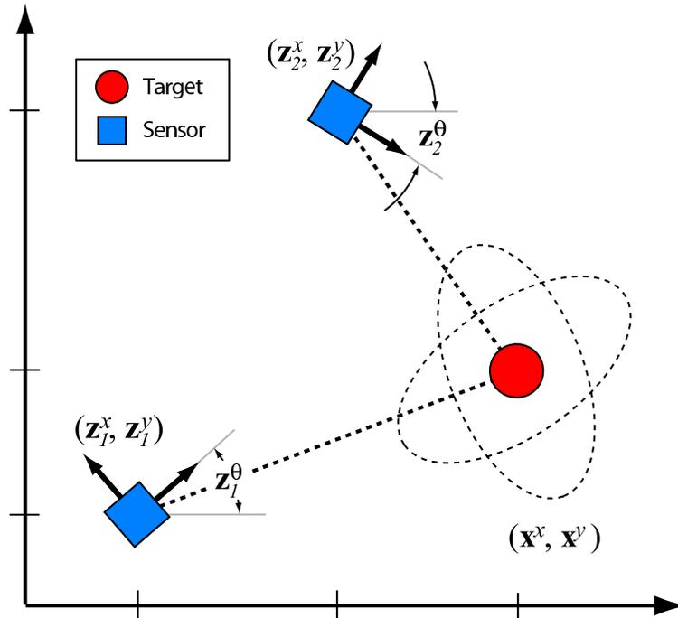
Figure 2.1: Illustration of the distributed target tracking problem. A team of  $M = 2$  mobile sensing platforms take range-and-bearing measurements of the target position in  $\mathbb{R}^2$ .
