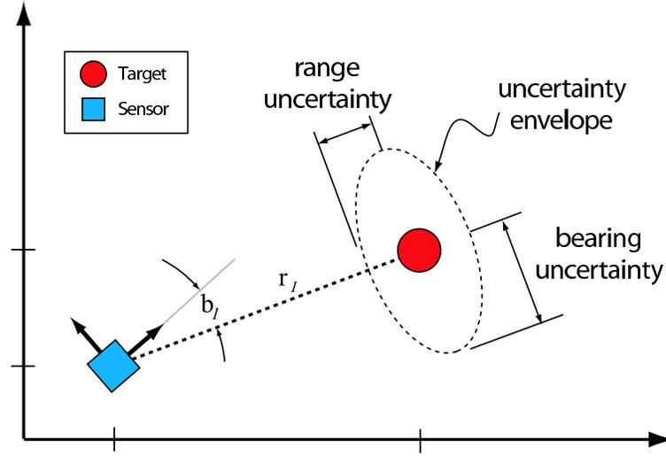
Figure 2.2: Schematic of the observation model, capturing the uncertainty in range-and-bearing measurements of the target's position in  $\mathbb{R}^2$ .
