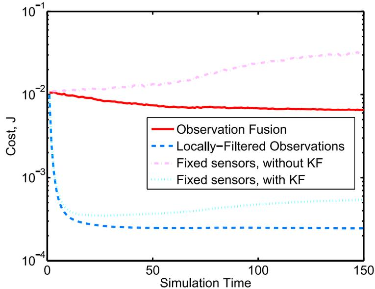
Figure 2.5: Evolution of the cost for an illustrative simulation run. Comparison of the algorithms shows that mobile sensors outperform stationary ones (i.e., have lower overall sensing uncertainty). Selection of the fusion approach (either sharing local observations or locally filtered estimates) is a design choice between performance and computation constraints.
