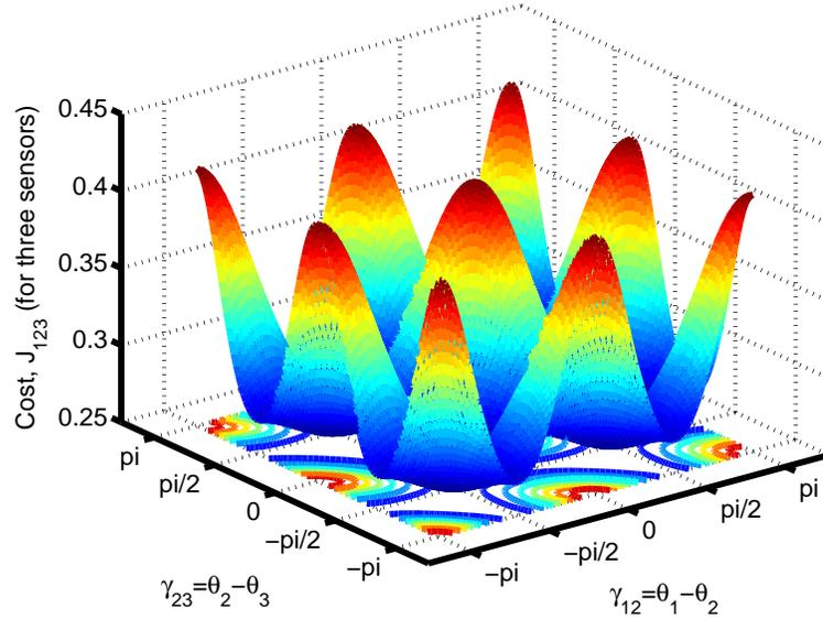
Figure B.2: Dependence of the cost function (for three sensors) on their relative bearings with respect to the target. Minimization of cost requires that agents be separated by  $\pm \frac{\pi}{3}$  (or by symmetry,  $\pm \frac{2\pi}{3}$ ) radians.
