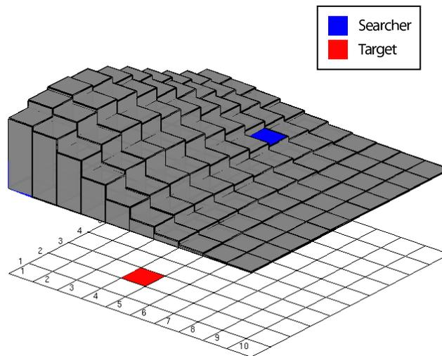
Figure 3.3: The search problem on a  $10 \times 10$  grid, with prior distribution modeled as a discretization of a Gaussian distribution with mean  $(1, 3)$  and covariances  $\sigma_i = 7$  and  $\sigma_j = 15$ . The initial positions of the searcher and target are  $(5, 8)$  and  $(4, 3)$ , respectively.
