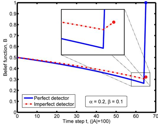
Figure 3.7: Effect of receiving a nonnull observation at  $t = 65$  on the evolution of the belief for the perfect and imperfect detector.
