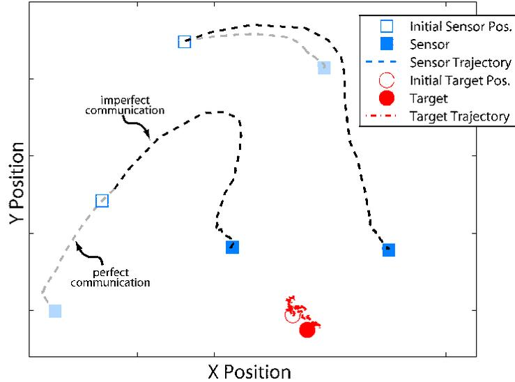
Figure 2.6: Two sensors track a randomly walking target: With imperfect communication (dark), or with perfect communication (light).
