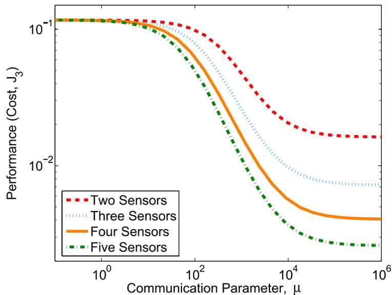
Figure 2.7: Sensing and communication performance tradeoff as a function of communication parameter,  $\mu$ .
