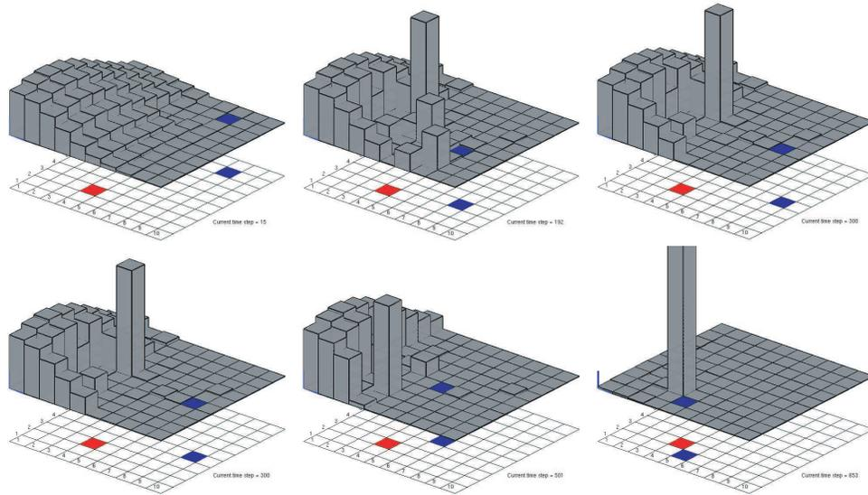
Figure 3.8: Illustration of belief probability distribution evolution for a single searcher randomly walking through the example search space to determine the presence of a stationary target. The random walk search strategy results in long times-till-decision but can be used as a limiting case in examining the performance of different search strategies.
