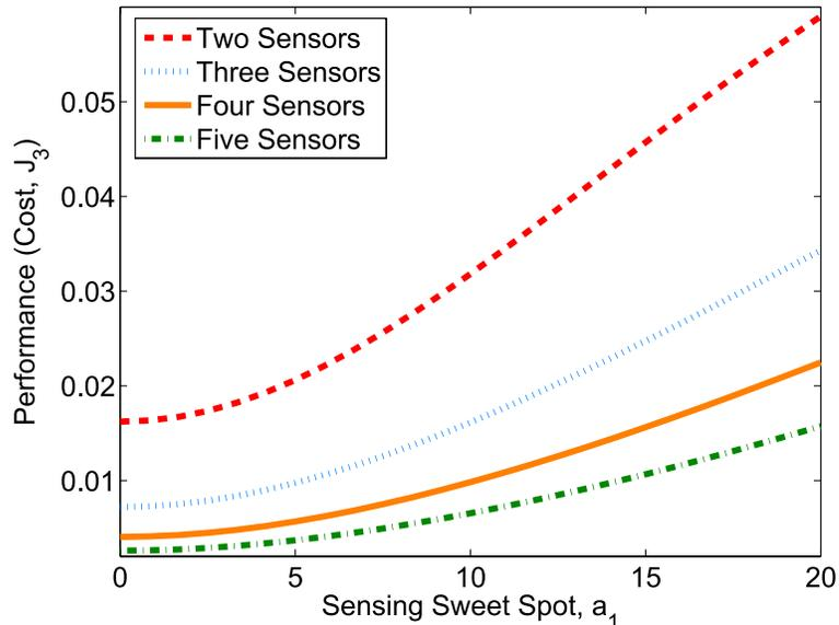
Figure 2.8: Sensing and communication performance tradeoff as a function of sensing sweet spot,  $a_1$
