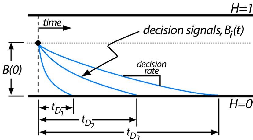
Figure 3.1: Schematic of the evolution of three decision processes, with varying values of time till decision. Feedback can be used to improve the performance, i.e., reduce the time until a decision is made.
