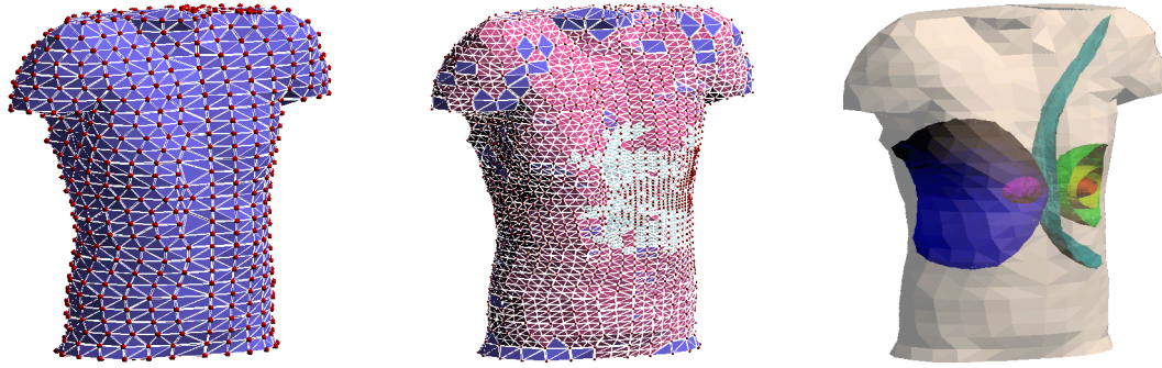
Figure 5.9: ECG field analysis example. On the left the initial grid; in the middle the refined discretization (four levels of substitution refinement). Red balls indicate active scaling functions, elements of different colors indicate the support of scaling functions on different levels. On the right, isocontours of the (adaptive) solution. Initial surface grid courtesy of the Center for Scientific Computing and Imaging, University of Utah.
