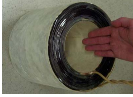
Figure 3.4: Photograph of the 13 cm bore, 0.4 T, 10 kW polarizing magnet used for polarizing protons in water in the PMRI experiments.
