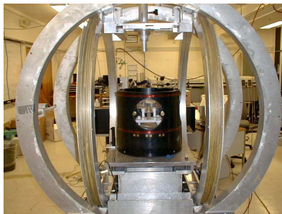
Figure 2.8: A photograph of the Helmholtz electromagnet at Caltech.
