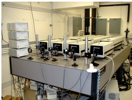
Figure 2.6: A photograph of the Ti-Sapphire lasers which were used for optical pumping at Caltech.
