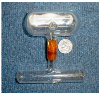
Figure 2.4: ^{129}\text{Xe} cell used for NMR and EPR polarimetry studies.
