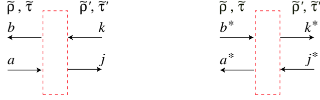
Figure 4.12: A two-port linear optical system can always be expressed in terms of four effective transmissivities and reflectivities, \tilde{\rho}' , \tilde{\tau}' (for fields entering from the right side), and \tilde{\rho} , \tilde{\tau} (for fields entering from the left side). By taking the complex conjugates of the field amplitudes and inverting their propagation directions, a new set of fields related by the same set of transmissivities and reflectivities is obtained.
