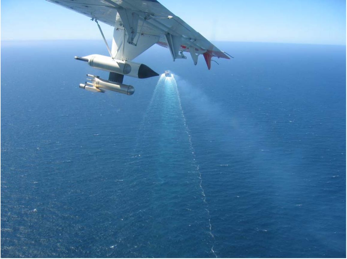
Figure 5.1: Photograph taken of the container ship from the cabin of the CIRPAS Twin Otter (the plane's wing tip is in the foreground) during the study. The exhaust plume is visible traveling with the mean wind at \sim 10^\circ angle to the heading of the ship, which can be inferred by the visible wake.
