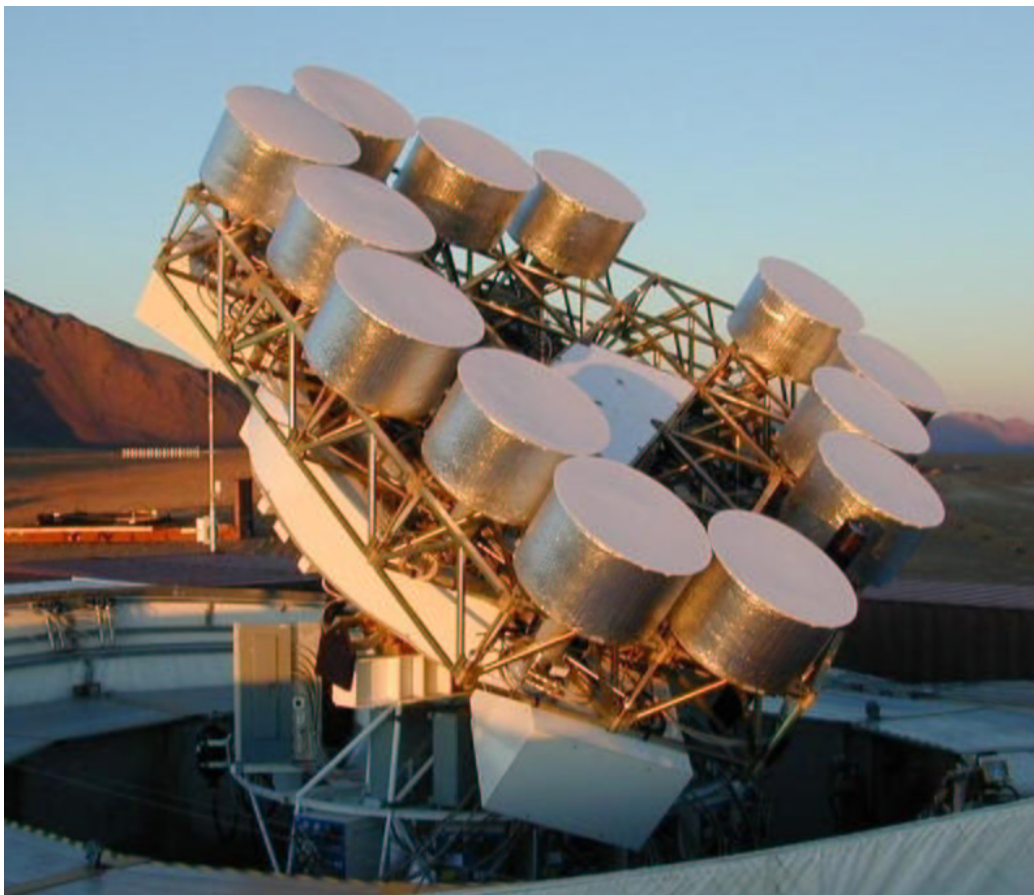
Figure 2.1: The Cosmic Background Imager at an altitude of 5080 m on the Chajnantor site in northern Chile. The 13 Cassegrain antennas have cylindrical shields which reduce crosstalk between the antennas. In this picture, the array is in the initial sparse configuration (configuration 1); in April 2000, the array was reconfigured to emphasize shorter baselines. The clamshell dome, seen open at the base of the telescope, is surrounded by shipping containers which contain living spaces, a control room, and laboratory and machine shop facilities. A pair of diesel generators provides power for the facility, and a cell phone with an amplified link ties the site to the project base camp in the nearby town of San Pedro de Atacama.
