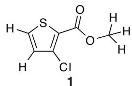
**Figure A.1.** Chemical structure of methyl 3-chlorothiophene-2-carboxylate (**1**)
