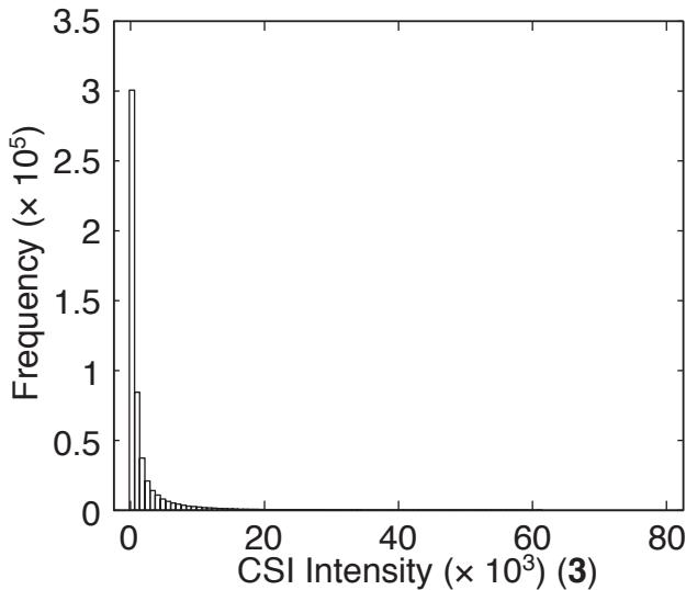
**Figure C.2.** CSI Intensity Histogram for polyamide 3
