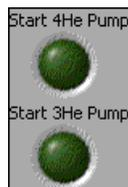
These two booleans are used to trigger pumping of the  $^4\text{He}$  and  $^3\text{He}$  stages.
