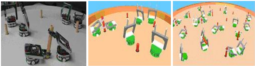
Figure 4.1: Left: Physical setup for the stick-pulling experiments. Center: Setup in the embodied simulator (4 sticks, arena of radius 40 cm). Right: Simulated Setup with 16 sticks and arena of radius 80 cm.
