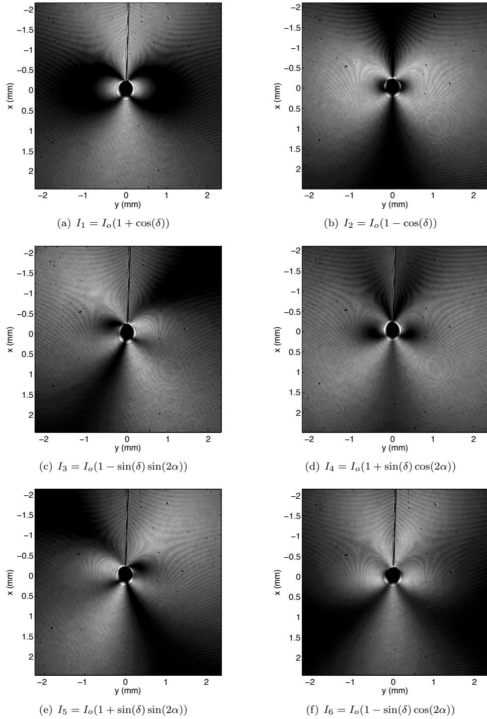
Figure 4.3: Experimental images from six-step phase-shifting photoelasticity for specimen HomC1 for  $K_I = 0.514 \text{ MPa}\sqrt{\text{m}}$  and  $K_{II} = 4.4 \text{ kPa}\sqrt{\text{m}}$ : Caustic shadows obscure the data at the crack tip due to the stress concentration, and the weak high density fringes overlaying the photoelastic fringes are due to the interference of the reflections from the front and back faces of the specimen.
