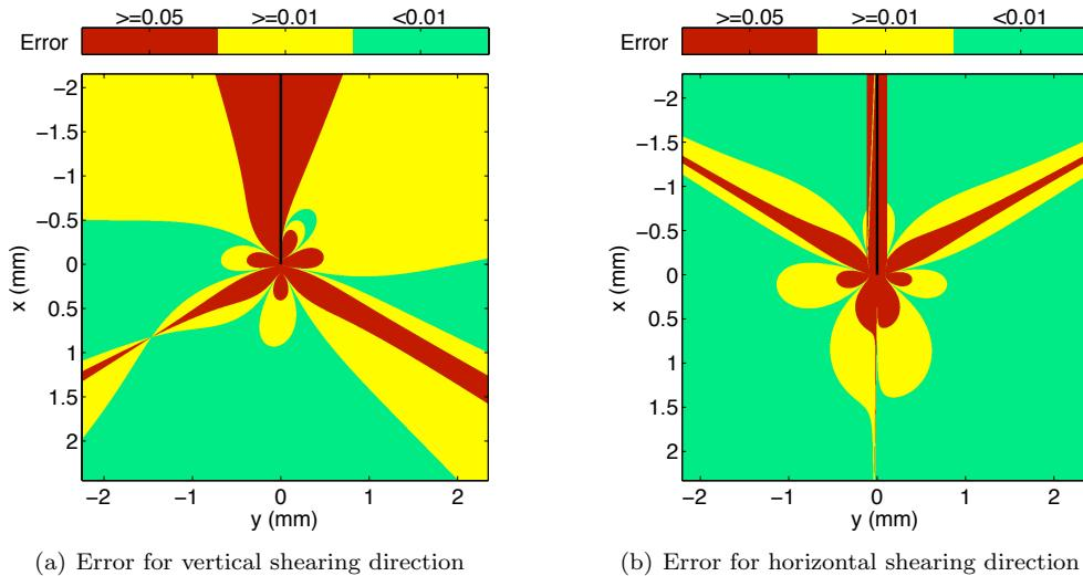
Figure 4.41: Theoretical error for CGS approximating the derivatives of  $\sigma_1 + \sigma_2$ , assuming  $K_I = 0.259$  MPa $\sqrt{\text{m}}$  and  $K_{II} = 5.0$  kPa $\sqrt{\text{m}}$  for the 4.6 mm  $\times$  4.6 mm field of view and lateral shearing distance of  $d_{shear} = 225$   $\mu\text{m}$  [Crack indicated in black]
