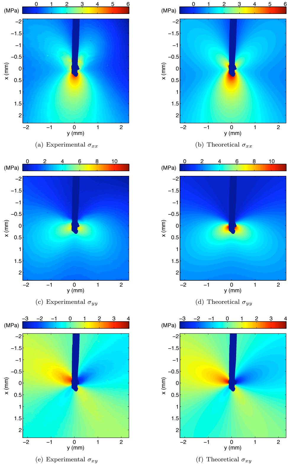
Figure 4.43: Experimental and theoretical data for the Cartesian stresses for specimen HomC1 for  $K_I = 0.259 \text{ MPa}\sqrt{\text{m}}$  and  $K_{II} = 5.0 \text{ kPa}\sqrt{\text{m}}$  with crack region masked in blue
