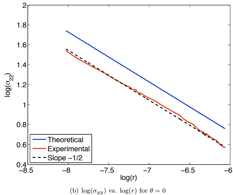
Figure 4.45: Experimental and theoretical data for  $\sigma_{yy}$  along  $\theta = 0$  for specimen HomC1 for  $K_I = 0.259 \text{ MPa}\sqrt{\text{m}}$  and  $K_{II} = 5.0 \text{ kPa}\sqrt{\text{m}}$ : The experimental data is slightly lower than the theoretical data, but with similar  $r^{-1/2}$  dependence seen by the near  $-1/2$  slope on the log-log plot of  $\sigma_{yy}$  versus  $r$ .
