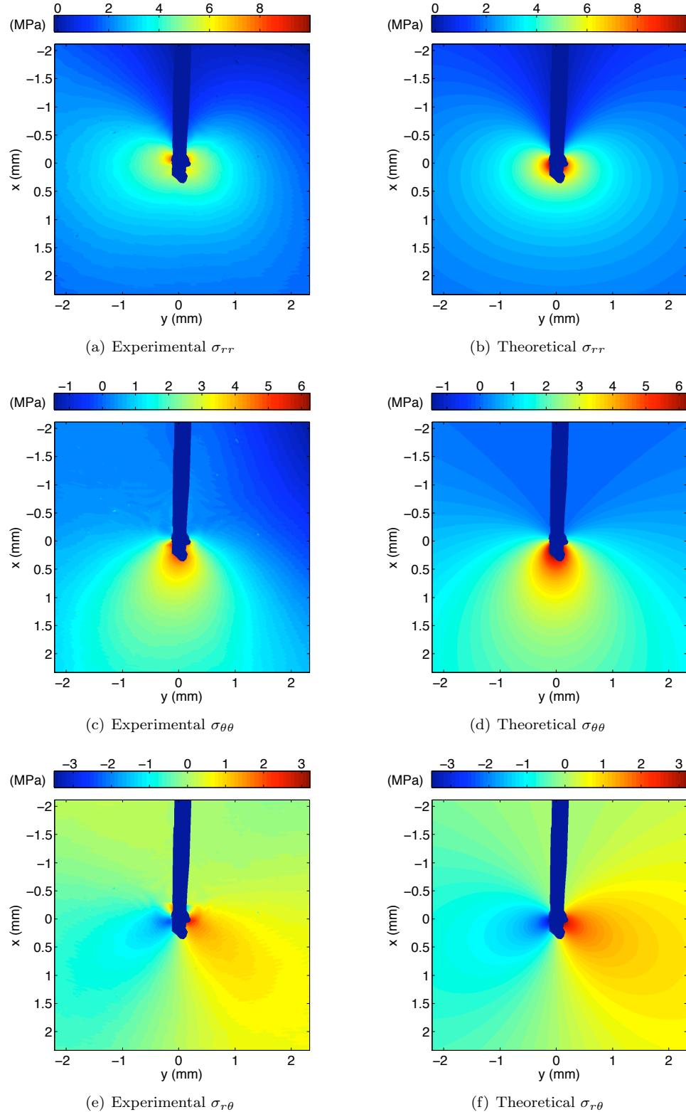
Figure 4.44: Experimental and theoretical data for the polar stresses for specimen HomC1 for  $K_I = 0.259 \text{ MPa}\sqrt{\text{m}}$  and  $K_{II} = 5.0 \text{ kPa}\sqrt{\text{m}}$  with crack region masked in blue
