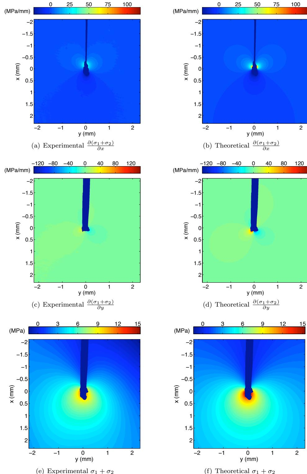
Figure 4.40: Experimental and theoretical data for the derivatives of  $\sigma_1 + \sigma_2$  and the experimental integrated  $\sigma_1 + \sigma_2$  for specimen HomC1 for  $K_I = 0.259 \text{ MPa}\sqrt{\text{m}}$  and  $K_{II} = 5.0 \text{ kPa}\sqrt{\text{m}}$  with crack region masked in blue
