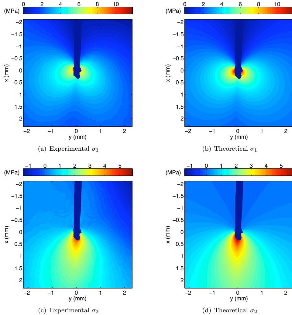
Figure 4.42: Experimental and theoretical data for the principal stresses for specimen HomC1 for  $K_I = 0.259 \text{ MPa}\sqrt{\text{m}}$  and  $K_{II} = 5.0 \text{ kPa}\sqrt{\text{m}}$  with crack region masked in blue
