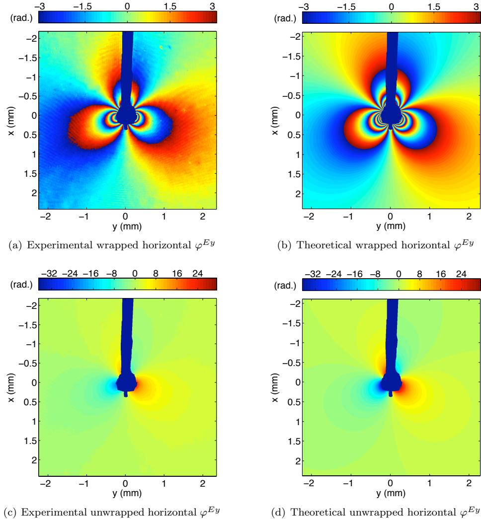
Figure 4.24: Experimental and theoretical  $\varphi^{Ey}$  data for horizontal CGS for specimen HomC1 for  $K_I = 0.514 \text{ MPa}\sqrt{\text{m}}$  and  $K_{II} = 4.4 \text{ kPa}\sqrt{\text{m}}$  with crack region masked in blue
