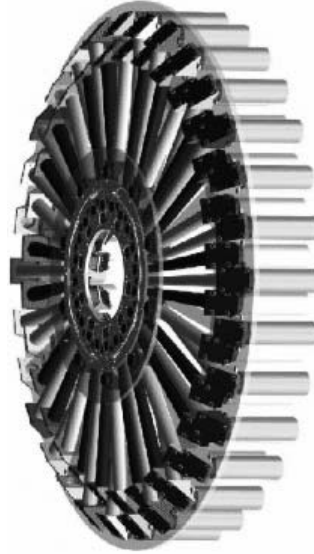
Figure 4.5: Light guide configuration.
