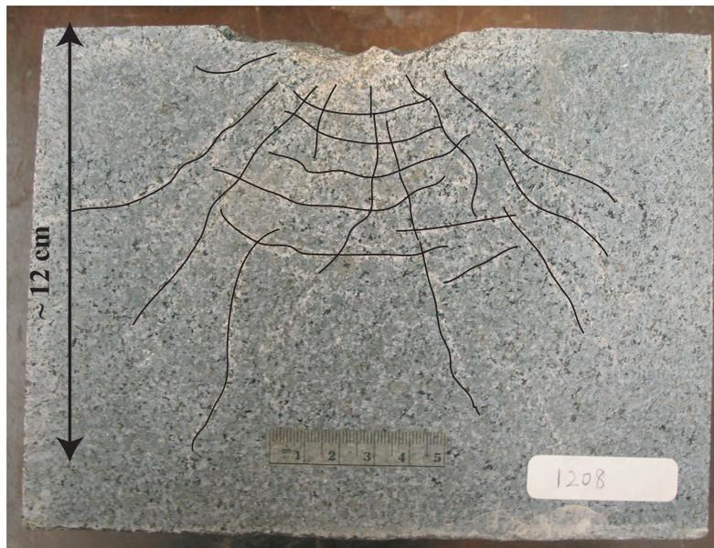
Figure 5.1: Shot 1208, granite impacted by  $\sim 25$  g lead ball (with sabot) at 800 m/s. Scale is 5 cm. (a) Top view showing impact crater. Also shown is cross section position for (b); (b) Cross section of target after being cut open. Tensile cracks extend to  $\sim 12$  cm for this case.
