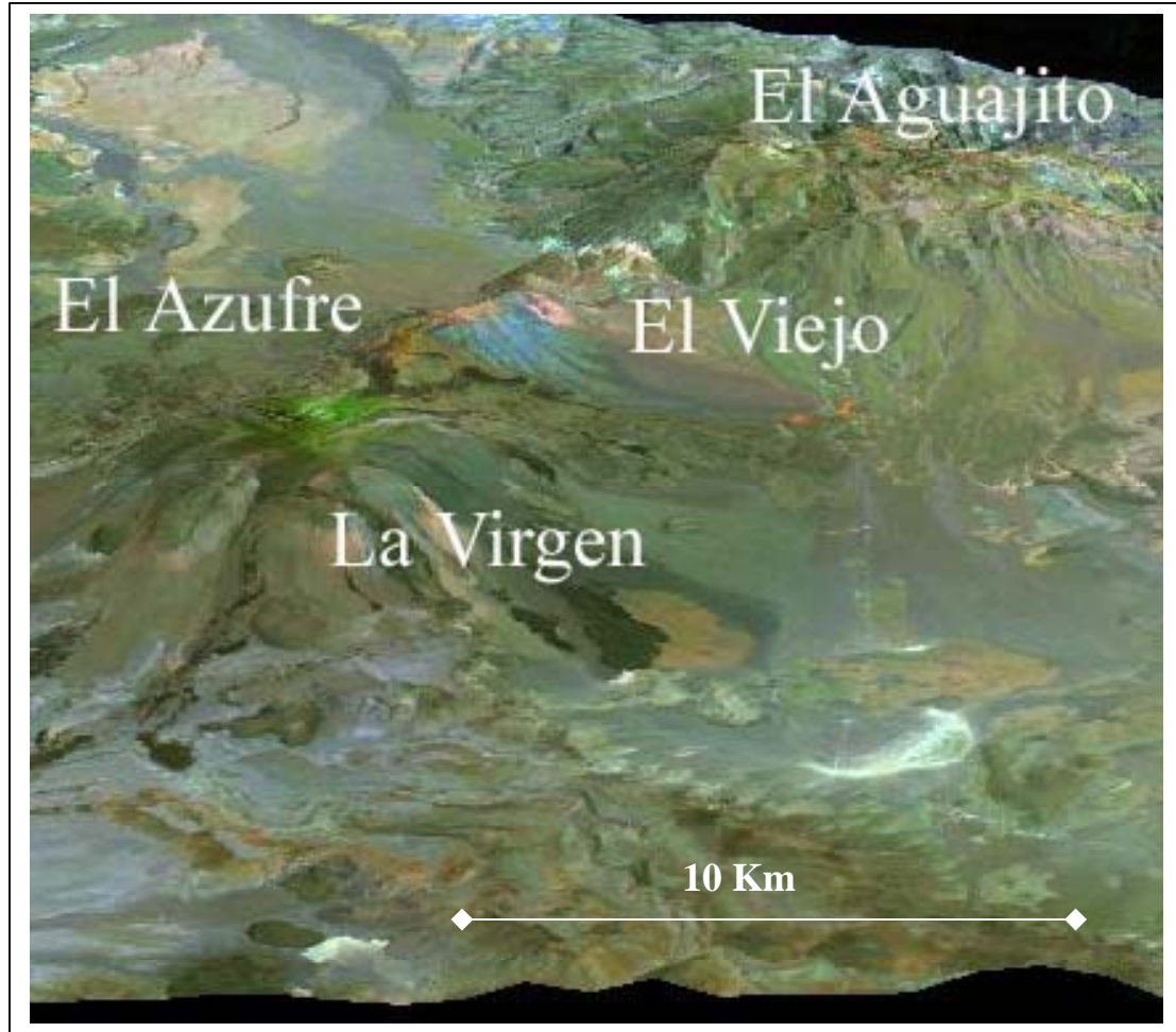
Figure 4. A Thematic Mapper image (Red: band 7, Green: band 4, Blue: band 1) of the Tres Vírgenes region, draped over a USGS 90 meter digital elevation model. Map datum and projection: NAD27 Mexico, UTM zone 12.
