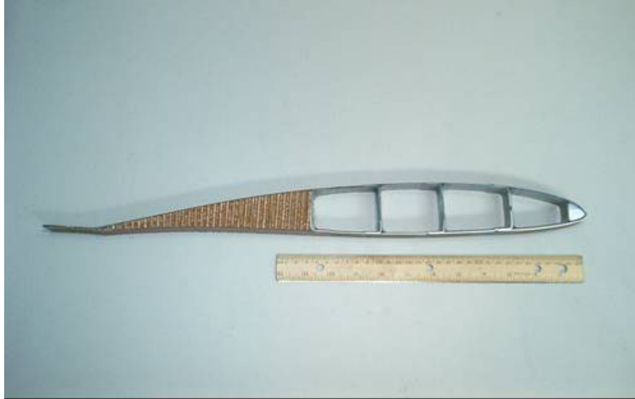
Figure 3.14: Cross section of the blade. For the example, the complex composite structure has been replaced by a homogeneous solid one.
