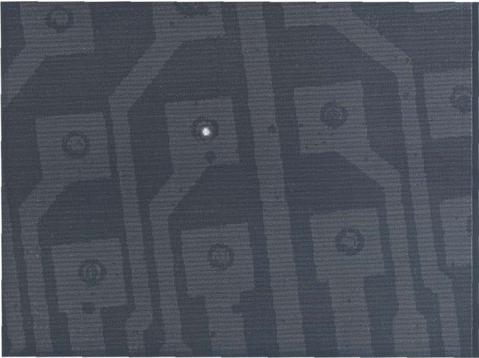
Figure 5.4. A higher magnification view of the 8x8 array with one laser operating.
