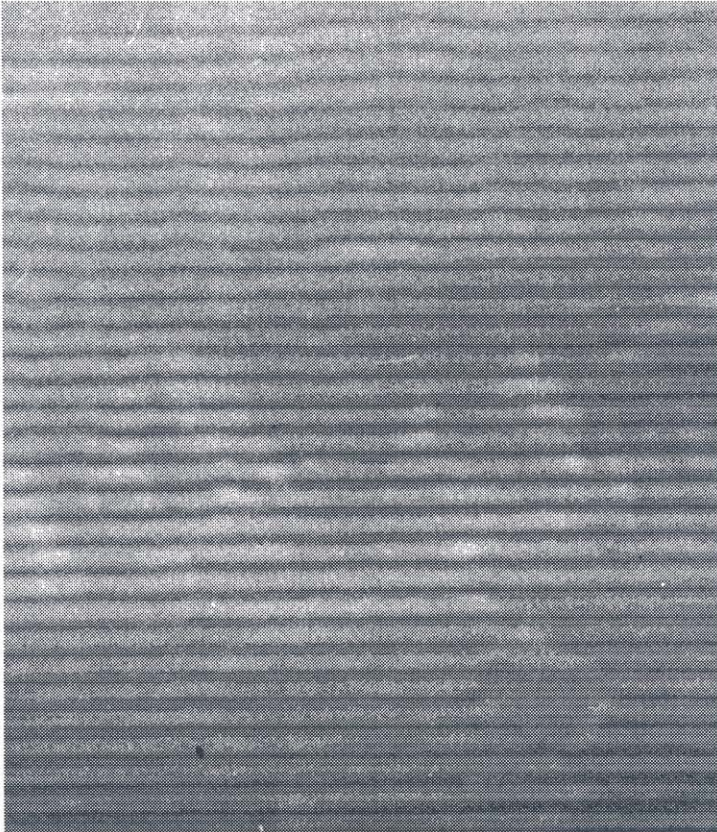
Figure 4.9. SEM micrograph showing a distributed Bragg reflector containing ternary AlGaAs layers. The roughness often seen in AlGaAs layers at low growth temperatures is visible.
