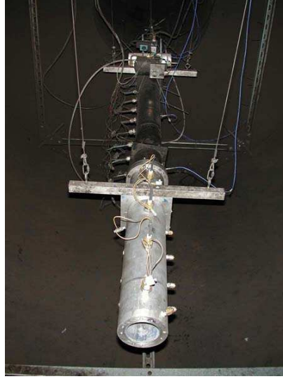
Figure 2.13: Photograph of the detonation tube with the straight extension (or 0°-0.6 m nozzle) installed.
