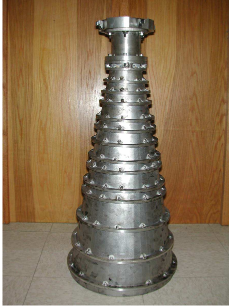
Figure 2.12: Photograph of 12°-0.6 m nozzle with a converging-diverging throat section installed.
