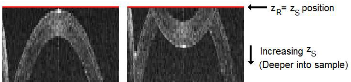
Figure 2.8: Mirroring example of the SDOCT image for two different reference arm positions. The change in the reference arm position of an intensity image (left) creates a mirrored image (right) in this case.
