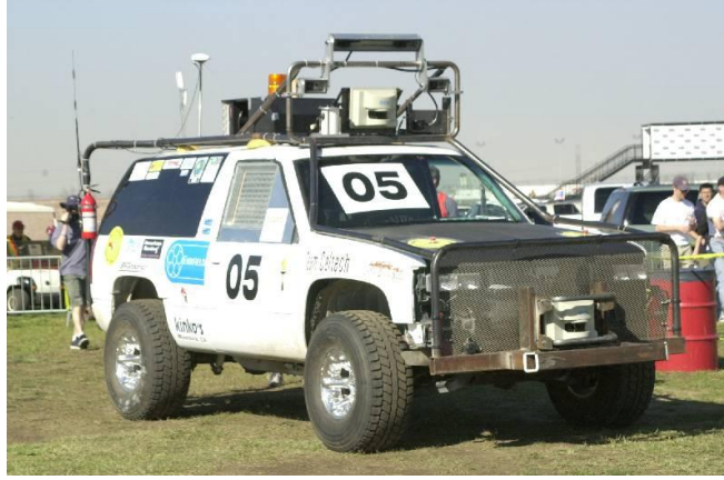
Figure 3.1. Bob, Team Caltech’s entry in the 2004 DARPA Grand Challenge, provides the test data for the results presented. Two stereovision camera pairs and a Sick LMS-2100 laser rangefinder are shown mounted above the cab; another Sick unit is mounted on the bumper. A Kalman filter achieves state estimates from differential GPS and IMU input data.
