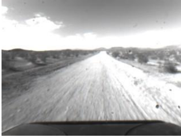
Figure 3.9. Visual forward image corresponding to position 2 of fig. 3.8. LADAR-based road-feature estimation has the advantage of insensitivity to lighting conditions such as long shadows, but is limited to a single look-ahead range. Computation times are significantly faster with LADAR feature extraction.
