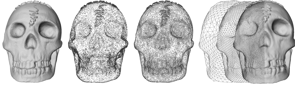
Figure 1.2: A 3d surface (left) is sampled by a number of points (center left). Connectivity information is added to the point cloud to form an irregularly triangulated mesh (center right). The connectivity between vertices can be simplified by resampling the geometry into a multi-resolution mesh with (semi-)regular connectivity (right).
