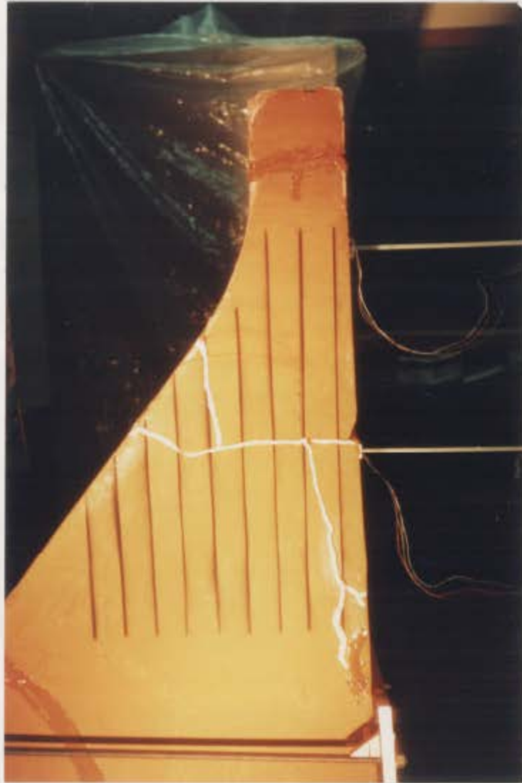
Figure 4.11: (a) Filmed side of monolithic model after initial cracking earthquake test.
